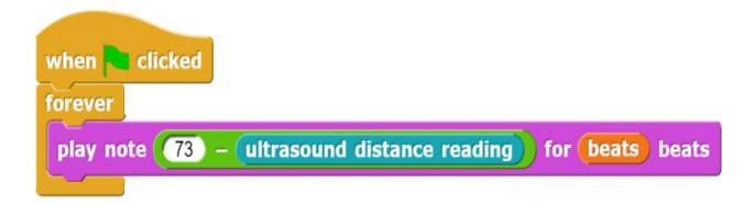
Script for controlling the ultrasound sensor and reproducing a specific note (left hand)
