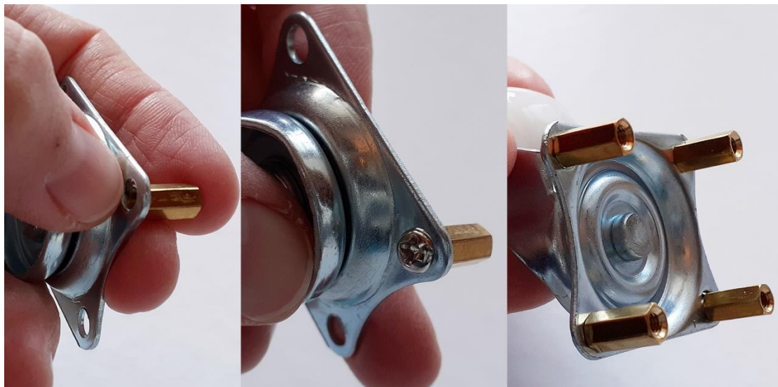
Figure 9: Assembling the caster. Left: attaching a spacer on the caster; Middle: Binding the spacer with a screw; Right: Binding all the spacers on the caster
