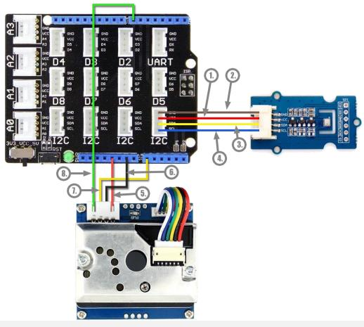
This diagram presents how the optical dust sensor is connected to Grove Base Shield.
