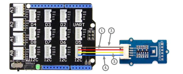
This diagram presents how the Grove Barometer Sensor module is connected to Grove Base Shield. For your convenience you are advised to use a 4-pin F-F Grove wire, and make sure that:
