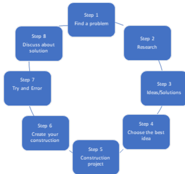
Figure 3: The Design process according the Design and Technology Curriculum (Cyprus Ministry of Education and Culture).
