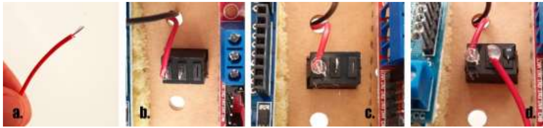
Figure 4: a. Revealing the wire of the cable using a wire stripper or a cutter; b. Folding the wire to the one pin of the switch; c. Gluing the wire by using hot glue gun; d. Gluing another wire that will connect the second pin of the switch to Shield's 5V
