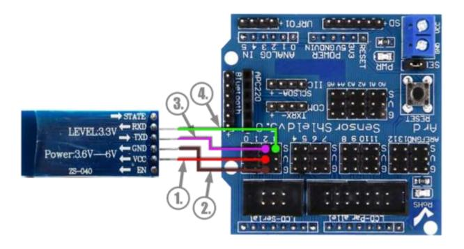
This diagram presents how the HC06 Bluetooth module should be connected to Arduino Sensor Shield, for the needs of Level 4 (namely, Controlling Remotely the DIY Automobile).
