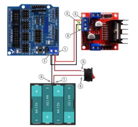
Connecting the battery holder and the switch to supply power
