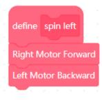
define spin right Left Motor Forward Right Motor Backward A number of consecutive commands are assigned to "spin left" procedure, instructing the DIY automobile to make a rather quick turn on the left, by setting the right motor to move forward and the left to move backwards.
