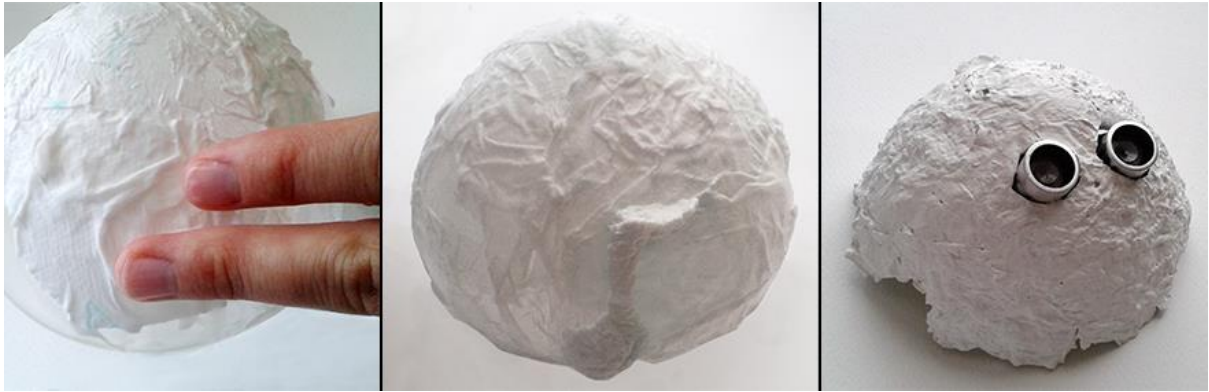
Figure 8 (Left) Placing the soaked piece of paper on the mold, (centre) waiting for the model to dry, (right) finished model
