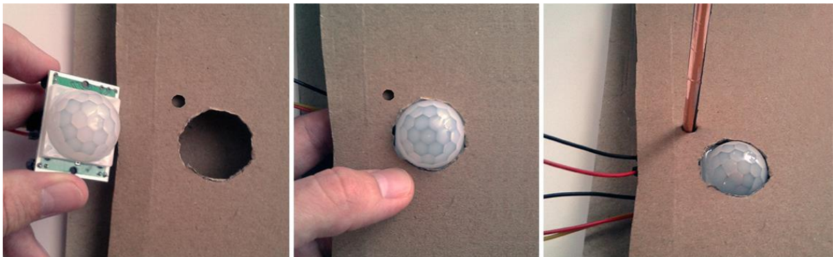
Figure 4: Embedding the PIR sensor and the straw on the base.
