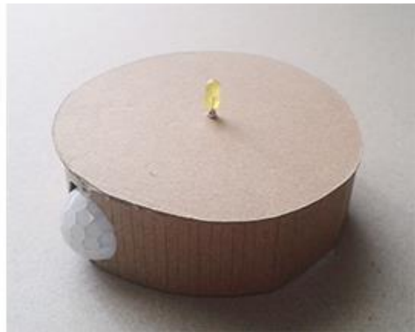
Figure 10: (Left) Gluing the stripe to the circle, (Right) Embedding the PIR sensor and the LED
