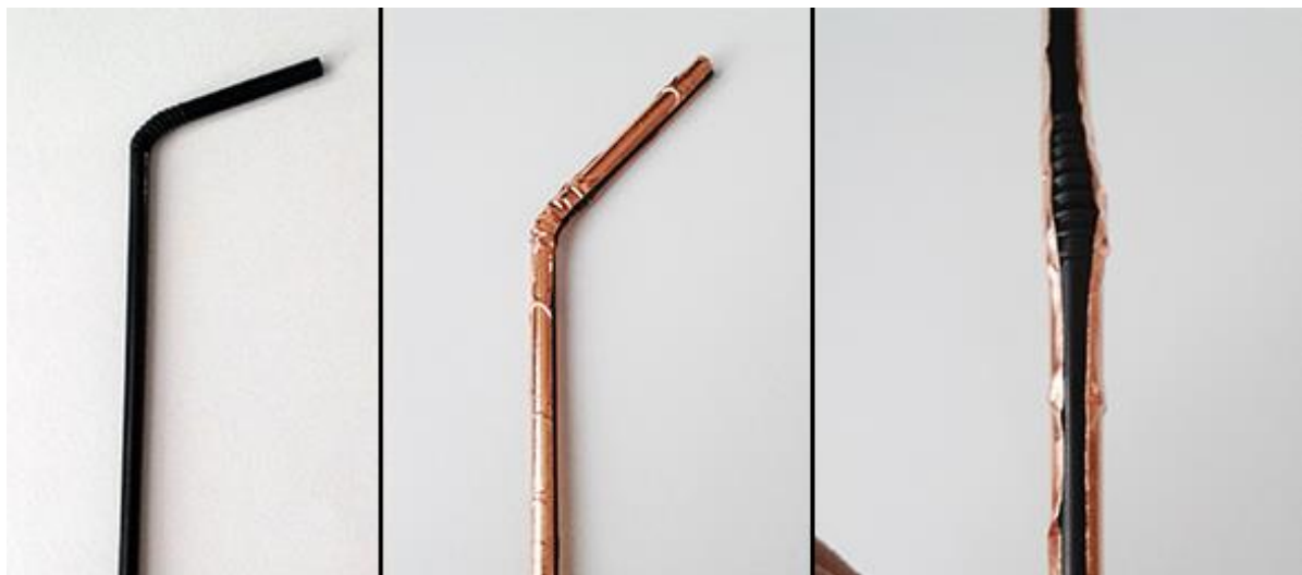
Figure 2: Covering the straw with the copper tape. Important note: When using copper tape, you should bear in mind that in case of overlapping, a short circuit will be created.
